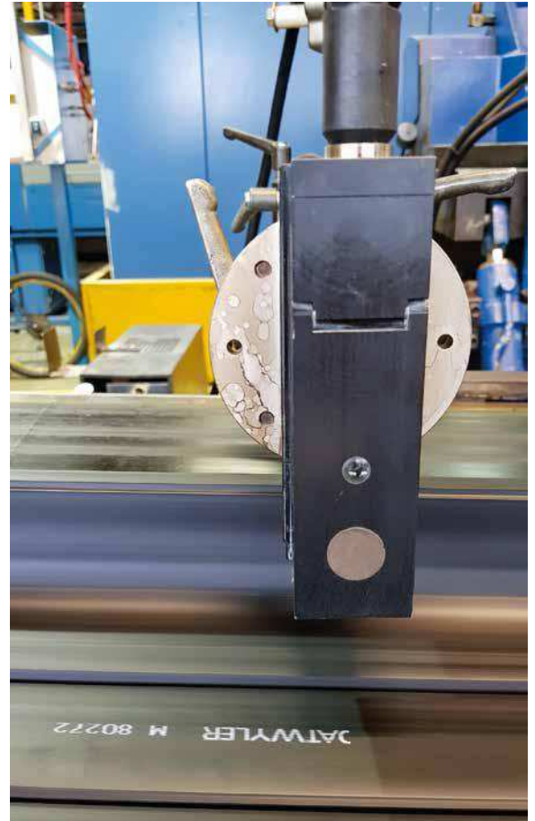
The alphaJET inkjet coding system adds markings to the profiles
